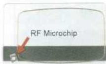
Transparent badge exposing laminated RF antenna loop & microchip
